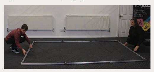
2. Lay the fabric over the frame. Begin clipping into place using the poppers around the frame, starting in the corners and work your way into the middle of the frame.
